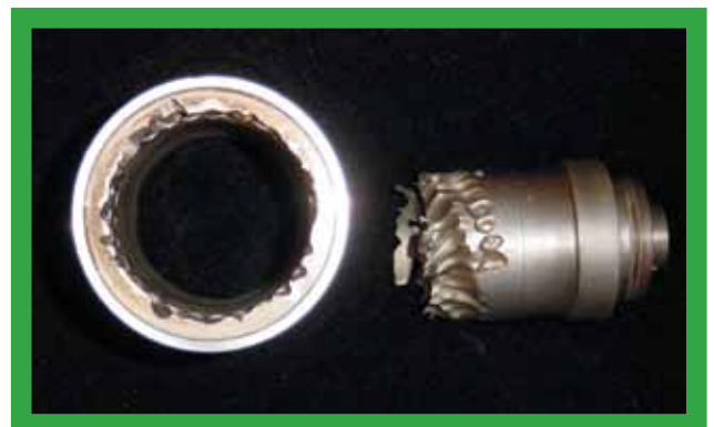
CAVITATION DAMAGED CAGE
