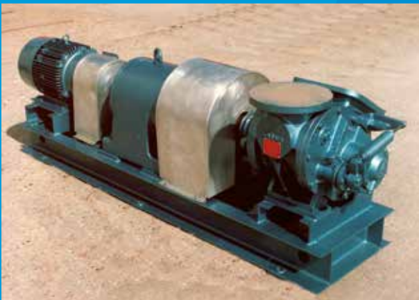
Magmo pump for the purpose of recirculating Massecuite to a Vertical Crystallizer.
