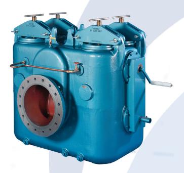
Cast Steel capable of operating at pressures up to 300 psig and temperatures of 200°C. They are fitted with a Stainless Steel 2mm perforated basket as standard, which can incorporate a removable mesh insert for fine filtration down to 300 mesh (50 micron). A pressure equalizing valve is fitted as standard and options include electrical changeover operation, differential pressure indication or control switch and replaceable mesh inserts from 20 to 300 mesh.
