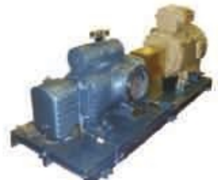
Used for tank to tank transfer in an oil storage terminal
