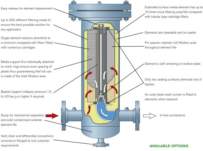
Dollinger has up to 200 filter media available to cover service applications such as alkaline solutions, organic liquids, water, weak acids, bases, oxidizing agents, lube oils etc
