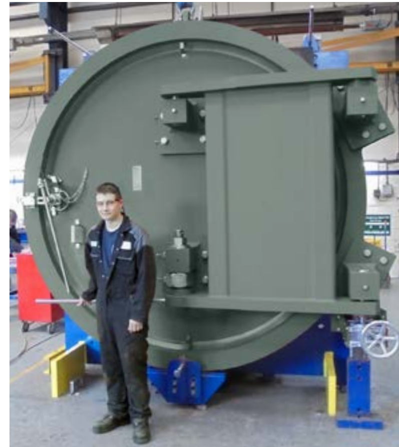
90" Horizontal Bandlock™2 Closure (90 barg) as supplied into the Middle East
