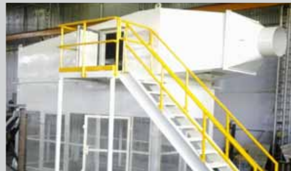
Air Separation Plant Two Stage Unit – 17,000 Nm 3 /hr
