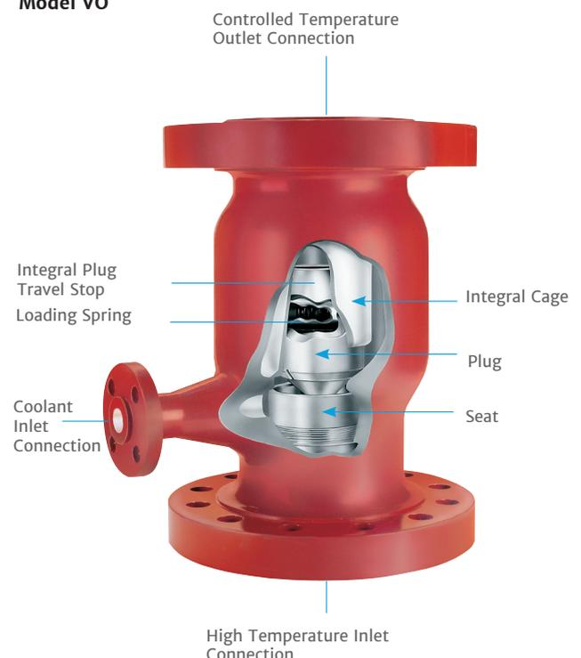
This pressure drop creates a relatively high velocity across the seat area, and it is at this point of low pressure constant velocity that the coolant is admitted into the vapor flow.
