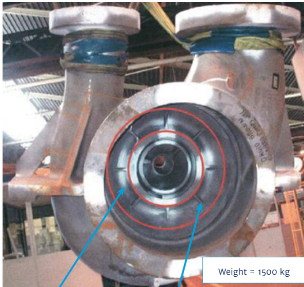
Casing cover with erosion resistant coating
