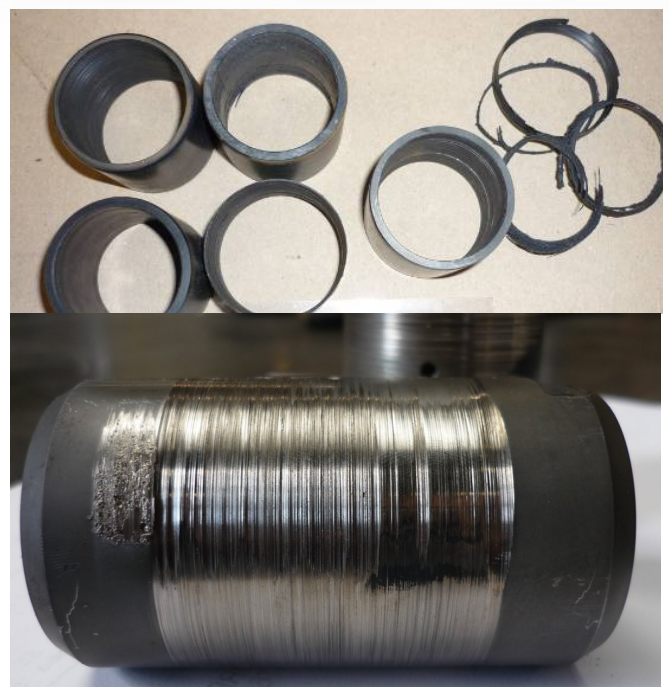
Impellers, PEEK bearings and bearing sleeves damaged
