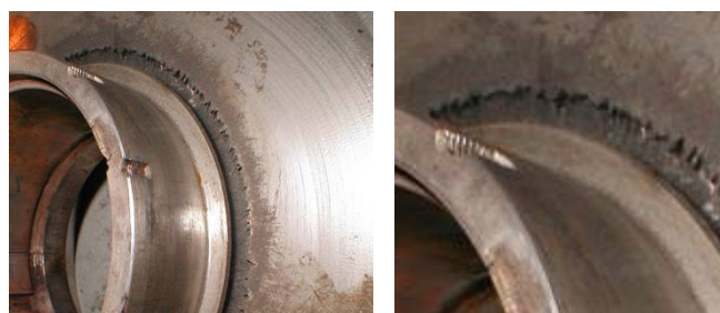
Damage to the back shrouds of impellers
