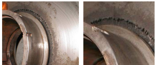
Damage to the back shrouds of impellers
