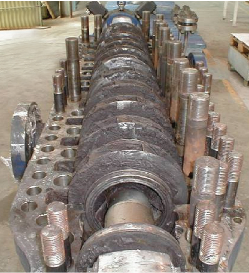
Image left: Erosion/scaling of pump parts
