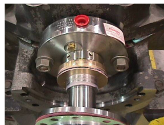
New mechanical seals
