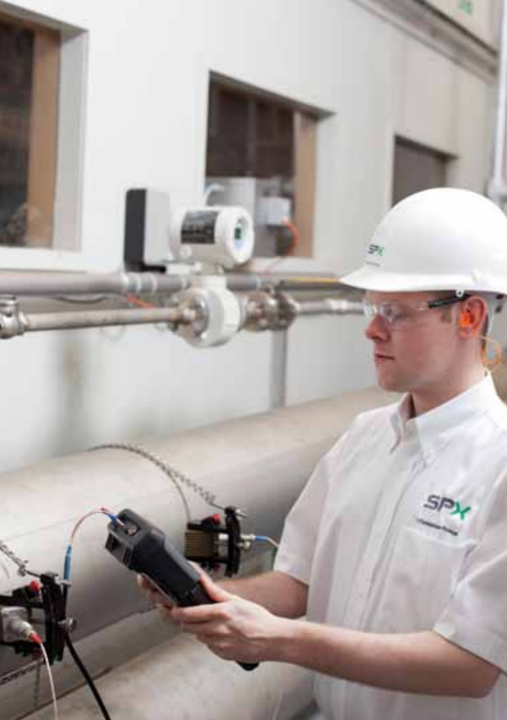
ABOVE - ON-SITE ULTRASONIC FLOW MEASUREMENT
