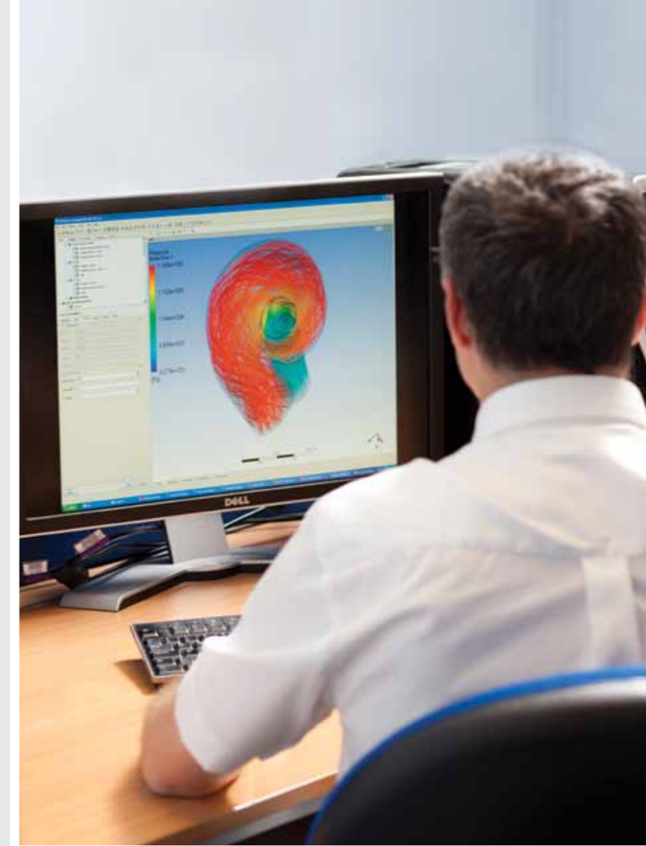
ABOVE - OPTIMISATION OF VOLUTE CASING EFFICIENCY USING CFD
