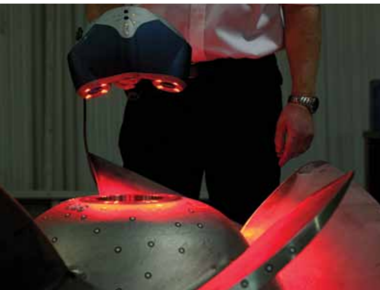
BELOW - 3D SCANNING AND RE-ENGINEERING PROCESS
