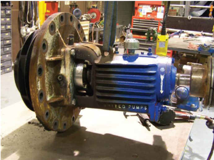
Existing bearing housing and cast cover
